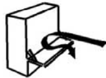
Figure 2.10: Example of counter measure for downwash - veranda on the base of the high building.
